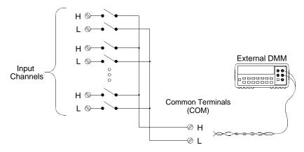
To control scanning with an external instrument, two control lines are provided. When the HP 34970A and the external instrument are properly configured, you can synchronize a scan sequence between the two.
