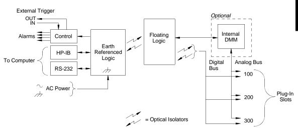
The earth-referenced and floating circuitry communicate with each other via an optically-isolated data link. The earth-referenced section communicates with the floating section to provide PC connectivity. The instrument is shipped with both an HP-IB (IEEE-488) interface and an RS-232 interface. Only one interface can be enabled at a time.
