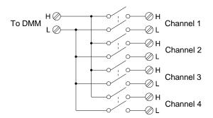
Note: If any channels are configured to be part of the scan list, you cannot close multiple channels; closing one channel will open the previously closed channel.
