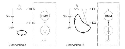
The measurement noise caused by injected current can be significantly reduced by setting the integration time of the internal DMM to 1 PLC or greater (see page 103 for a discussion of integration time).
