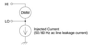
With *Connection A* (see below), the injected current flows from the earth connection provided by the circuit to the LO terminal of the internal DMM. This configuration adds no noise to the measurement. However, with *Connection B*, the injected current flows through the resistor R thus adding noise to the measurement. With Connection B, larger values of R will make the problem worse.
