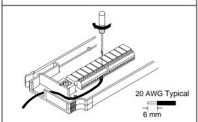
3 Route wiring through strain relief.
