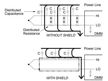
Common mode noise can dramatically affect the internal DMM. A typical thermocouple output is a few millivolts and a few millivolts of common mode noise can overload the input to the internal DMM.
