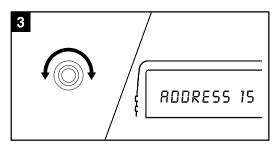
**3** Rotate the knob to view the choices on this level of the menu. When you reach the end of the list, rotate the knob in the opposite direction to view all of the other choices.
