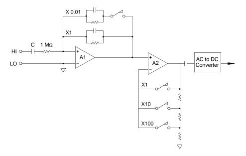
The first stage implements a high input impedance (1  $M\Omega$ ) switchable compensated attenuator. The second stage provides variable-gain signal amplification to scale the input to the ac converter to the full-scale level. Any residual dc offset from the attenuator and amplifier stages is blocked by a capacitor.
