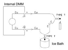
The T-type thermocouple is a unique case since one of the conductors (copper) is the same metal as the internal DMM's input terminals. If another type of thermocouple is used, two additional thermocouples are created. For example, take a look at the connections with a J-type thermocouple (iron and constantan):
