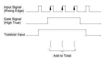
• Using the hardware jumper labeled "Totalize Threshold" on the module, you can control the threshold at which an edge is detected. Move the jumper to the "AC" position to detect changes through 0 volts. Move the jumper to the "TTL" position (factory setting) to detect changes through TTL threshold levels.
