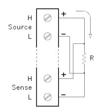
Channel *n* (source) is automatically paired with Channel *n+10* (sense) on the HP 34901A or Channel *n+8* (sense) on the HP 34902A.
