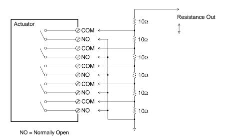
In the above diagram, the resistance is  $60\Omega$  when all of the actuator channels are open (not connected to COM). Note that when the actuator channels are open, as shown above, the normally-closed contacts (not shown above) are connected to COM. Values from  $10\Omega$  to  $50\Omega$  are selected by closing the appropriate channel(s) on the module.
