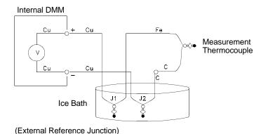
This circuit is the best solution for accurate thermocouple connections.
