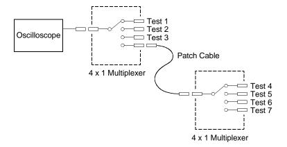
On the HP 34905A ( $50\Omega$ ) and HP 34906A ( $75\Omega$ ) RF multiplexers, you can close only one channel per bank at a time; closing one channel in a bank will open the previously closed channel. These modules respond *only* to the CLOSE command (OPEN does not apply). To open a channel, send the CLOSE command to another channel in the same bank.
