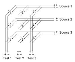
Any one of the signal sources can be connected to any one of the test inputs. Be aware that with a matrix, it is possible to connect more than one source at the same time. It is important to make sure that dangerous or unwanted conditions are not created by these connections.
