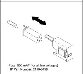
**3** Rotate the line-voltage selector until the correct voltage appears in the window.
